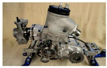
Assembled using all brand new parts, including 2-piece head, inlet assembly, 41.5mm Viper/Mikuni TMX carb, Honda generator, 2-curve programmable digital ignition, Mikuni DF-52 pump, inverted gearchange assembly, full exhaust inc. carbon silencer and airbox
